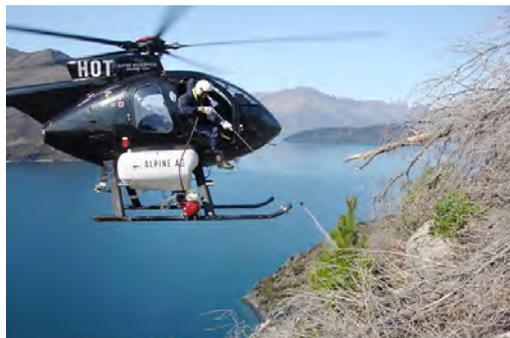
Figure 3. Aerial application of herbicide using a wand.
