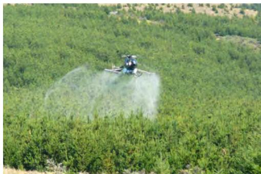
Figure 4. Aerial boom spraying a dense stand of wilding conifers.
