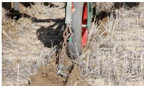
Figure 2. Banding nozzle to apply herbicides and ring harrow on the press wheels.
