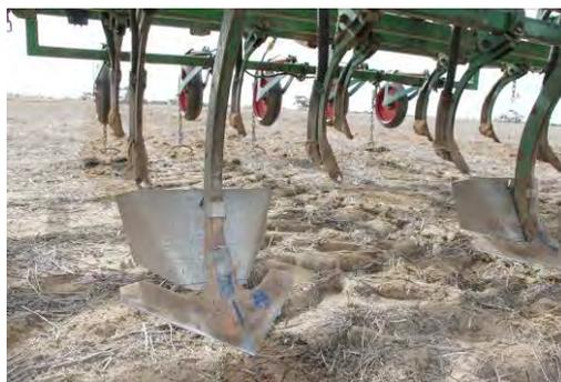
Figure 3. Soil scraper plate behind sweep points.
