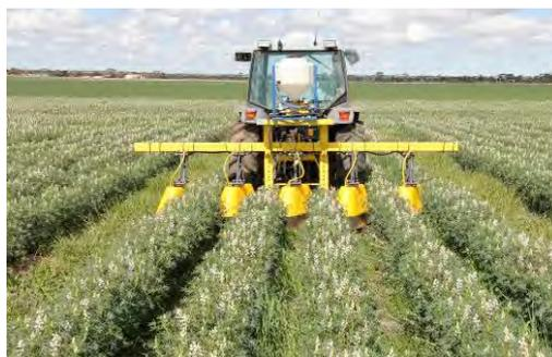
Figure 4. Shielded sprayer between rows 20-8-2013.
