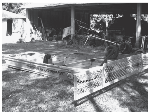
Figure 3. Aquadozer fitted with wings.
